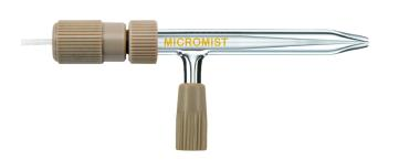
The novel design of the high efficiency nebulizer used in the Glass Expansion single-cell sample introduction system uses a low argon gas flow to provide high nebulization efficiency without rupturing the cell walls.
