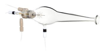
Conventional ICP-MS spray chambers have low transport efficiencies (< 5%) and filter out larger droplets (>5 $\mu$ m) preventing a high percentage of cells from entering the plasma. As most cell lines of interest are larger than 5 $\mu$ m, the spray chamber design for single cell analysis is different from conventional ICP-MS spray chambers.
